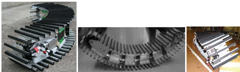
Fig. 8. Flexible Mono-tread Mobile Track (FMT). Lateral flexion (the left), retro-flexion (the middle) and twisting (the right)
