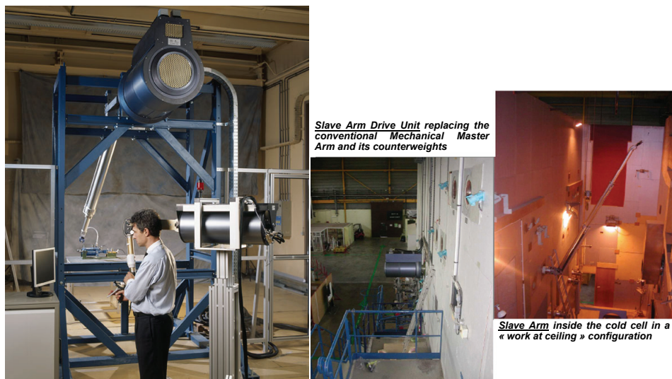
Fig. 11. The MT 200 TAO (CEA/ AREVA) developed for AREVA La Hague hot-cells.
