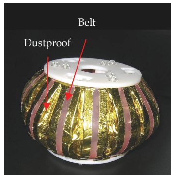
Fig. 27. Expansion belts and dustproof covering
