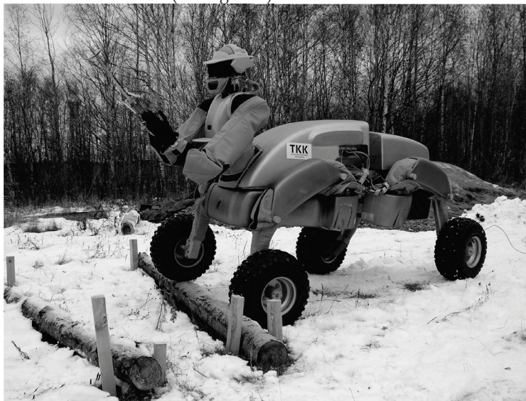
Fig. 3. The WorkPartner service robot seen here in winter on a test track, negotiating obstacles.
